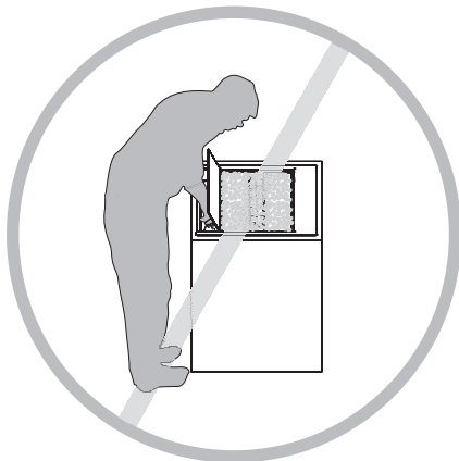
NEVER LEAN OVER FIREPIT WHEN LIGHTING BURNER
